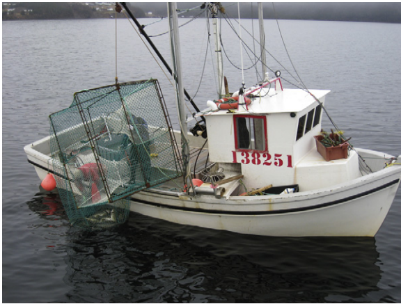
Fig. 5. A Newfoundland collapsible cod pot is being hauled onboard. Courtesy of Philip Walsh, Fisheries and Marine Institute, Memorial University, Canada.
